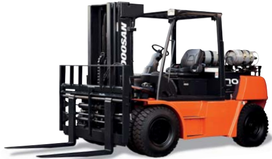
G50S / G60S / G70S-5 11,000lb(5,000kg) 13,500lb(6,000kg) 15,500lb(7,000kg) LP Gas ; Pneumatic Tire
